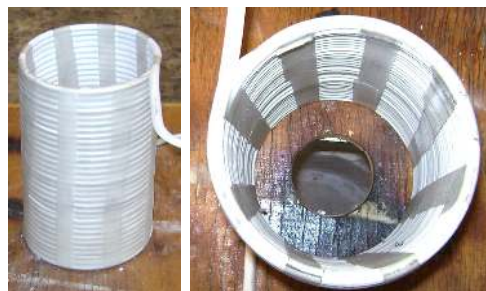
Figure 3.3-32 turn 'long' induction coil #4, 132 mm average diameter, 218 mm long, (D_{cs}/l)=0.60 [Supplement 3]. See Table 3 for details.
