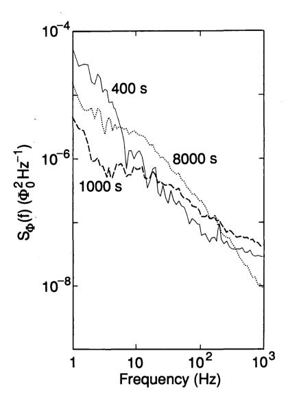
FIG. 8-5. Noise spectral density  $S_{\Phi}(f)$  vs. frequency for TCBCO(1) at three different times after cooling to 77 K in B = 0.1 mT. Measurements made after field was removed at t = 0: solid spectrum, t = 400 s; dashed spectrum, t = 1000 s; dotted spectrum, t = 8000 s. Increasing smoothness of spectra with increasing t is an artifact caused by longer averaging times.
