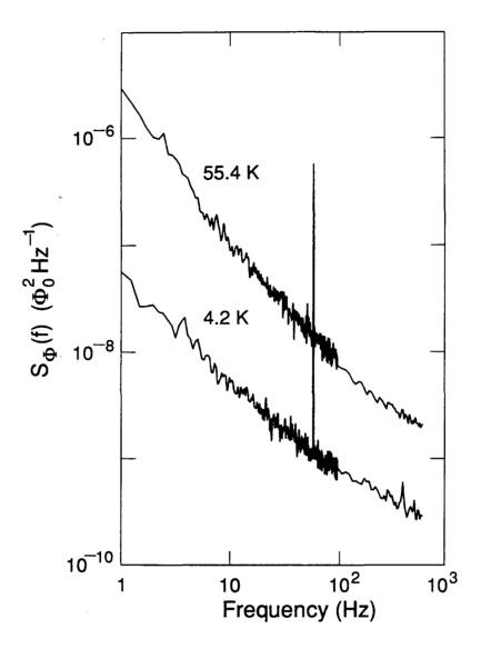
FIG. 6-2. Total noise power vs. frequency for transformer T2 at two temperatures in ambient field ( $B < 1\mu$ T). Noise in SQUID computed according to Eq. 2-1. Spike is 60 Hz pickup. Flattening at high frequencies caused by Johnson noise from normal metal components of apparatus.
