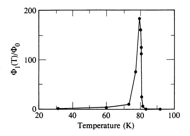
FIG. 8-4. Flux creep rate  $\Phi_1$  in units of the flux quantum vs. temperature for YBCO(1) after cooling in B = 1 mT. Greatest creep rate was measured at 79 K, well below  $T_c = 85$  K. Curve is a guide to the eye.
