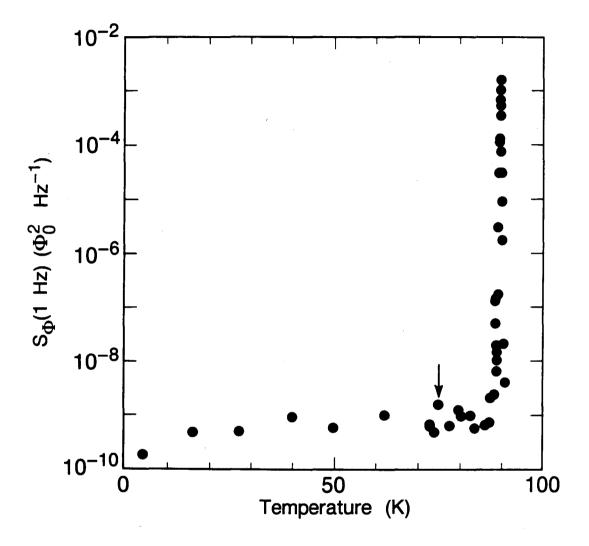
FIG. 4-5. Flux noise  $S_{\Phi}(1 \text{ Hz})$  vs. temperature for YBCO(3). Values below  $8 \times 10^{-10} \Phi_0^2/\text{Hz}$  include large contributions from the measuring system, and therefore represent upper limits on noise from the film. A significant and reproducible maximum in noise from the film occurs near 75 K (arrow), and a large peak at  $T_c = 89.8$  K.
