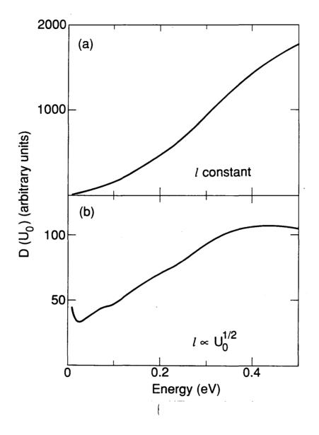
FIG. 5-5. Density of zero-temperature activation energies  $D(U_0)$  vs. energy  $U_0$  for a-axis sample YBCO(6) according to two models of the hopping distance  $\boldsymbol{\ell}$ . Both models employ  $\tau_0 = 10^{-11}$  s and  $\beta(T) = (1-t^4)/k_BT$ , and give  $D(U_0)$  in the same arbitrary units as Fig. 5-3. (a) Constant  $\boldsymbol{\ell}$ , generated by Eqs. (5-5) and (5-6). (b)  $\boldsymbol{\ell} \propto U_0^{1/2}$  from Eqs. (7-13) and (7-14).
