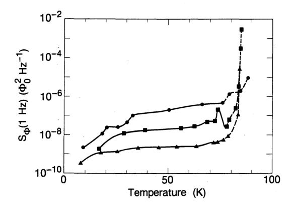
FIG. 5-1. Spectral density of flux noise at 1 Hz vs. temperature below  $T_c$  for three samples: squares, YBCO(1); triangles, YBCO(2); circles, BSCCO(1). SQUID noise has been subtracted. All data points show a 1/f-like noise power spectrum. Curves are piecewise cubic interpolants used to calculate m(T) (solid and dashed segments) and  $D(U_0)$ (solid segment only).
