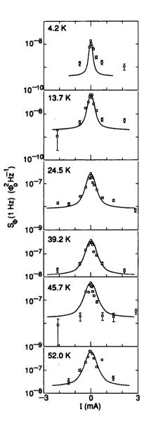
FIG. 7-2. Noise power  $S_{\Phi}(1 \text{ Hz})$  in SQUID vs. current in transformer T1 for six temperatures. Points are experimental data, from which the least noise measured at each temperature has been subtracted to remove background. Curves are the prediction of Eqs. (6-2) and (7-3) with indirect noise transfer function from Eq. (6-1). Central peak is due to input coil, shoulders to pickup loop.
