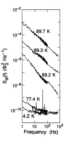
FIG. 4-4. Spectral density  $S_{\Phi}(f)$  of flux noise in YBCO(3) at five temperatures. At 4.2 K, the observed noise can be attributed to the SQUID measuring system; the SQUID contribution is significant at temperatures up to 87 K. Spikes are from 60 Hz pickup and microphonics.
