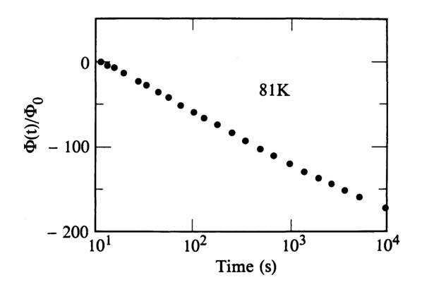
FIG. 8-3. Change in flux linking the SQUID in units of the flux quantum,  $\Phi(t)/\Phi_0$ , vs. time for YBCO(1) at 81 K. Sample was cooled through  $T_c$  in a magnetic field of 1 mT. Measurement made in zero applied field, and t = 0 is time at which the field was removed.
