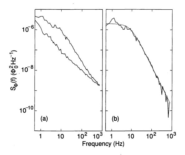
FIG. 3-6. Spectral densities of noise from BSCCO(2) at 50.6 K, referred to sample as in Eq. (2-2). (a) Total noise after positive-going (lower spectrum) and negative-going (upper spectrum) magnetic field increment. (b) Heavy curve, difference of spectra in (a); light curve, Lorentzian from Eq. (3-2) fitted with two free parameters:  $\tau = (\tau_1^{-1} + \tau_2^{-1})^{-1} = 18$  ms and  $(2\tau\Delta\Phi)^2/(\tau_1 + \tau_2) = 2 \times 10^{-6} \Phi_0^2/\text{Hz}.$
