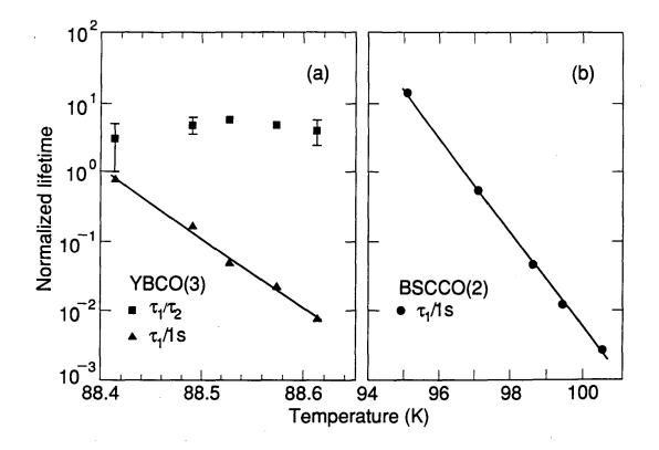
FIG. 3-3. Lifetimes vs. temperature for (a) YBCO(3) and (b) BSCCO(2). Solid lines are least-squares fits of Eq. (3-1) to  $\tau_1(T)$ assuming  $U(T) = U_0(1-t^4)$  and  $\tau_{A1} = 10^{-11}$  s. Fitting parameters are given in Table 3-2.
