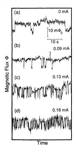
FIG. 7-4. Flux through SQUID vs. time generated by transformer T2 at 45 K for four different values of the circulating current I: (a) 0 mA, (b) 0.09 mA, (c) 0.13 mA, (d) 0.18 mA. Zeros of axes are arbitrary; traces are displaced for clarity.
