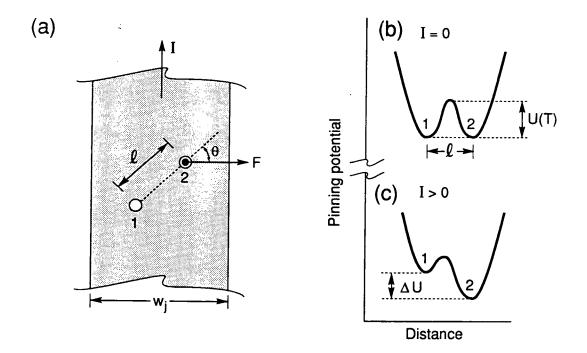
FIG. 7-3. (a) Schematic of single hopping process in transformer line of width  $w_j$ . Current *I* exerts force *F* on vortex which hops distance lbetween pinning sites 1 and 2. Scale of l exaggerated. (b) Schematic pinning potential for I = 0; (c) for I > 0.
