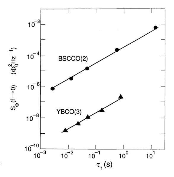
FIG. 3-4. Noise power on low-frequency plateau  $S_{\Phi}(f \rightarrow 0)$  vs. down-state lifetime  $\tau_1$  for two samples. Triangles, YBCO(3); circles, BSCCO(2). Noise in SQUID computed according to Eq. 2-1. Lines are least-squares fits with unit slope.
