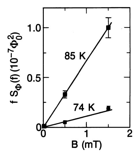
FIG. 8-1. Noise power  $f S_{\Phi}(f)$  for YBCO(3) at two temperatures as a function of the magnetic field B in which the sample was cooled (3 Hz  $\leq f \leq 30$  Hz). Lines are guides to the eye which intercept the origin.
