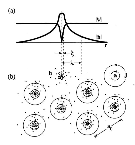
FIG. 1-1. Mixed state of a Type-II superconductor. (a) Amplitude of GL order parameter  $|\psi(r)|$  and local field |h(r)| as functions of radius raround an isolated vortex, after Fig. 5-1 of Ref. [79]. I follow the convention of de Gennes [80] in using h to denote the microscopic value of the magnetic induction B. (b) Sketch of triangular Abrikosov vortex lattice looking along direction of magnetic field, indicating flux density, circulating current J, and lattice constant  $a_0$ .
