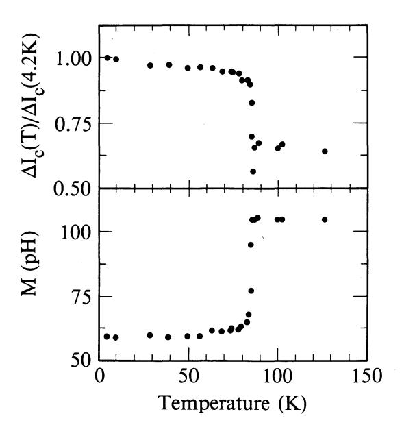
FIG. 2-5. Temperature dependence of SQUID parameters for sample YBCO(1). Upper graph, normalized modulation amplitude  $\Delta I_c(T)/\Delta I_c(4.2 \text{ K})$ ; lower graph, mutual inductance *M* between the SQUID and the feedback coil.
