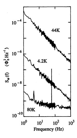
FIG. 4-1. Power spectra of total flux noise measured in sample YBCO(5) at three temperatures. The spectrum at 80 K shows noise from the SQUID, 60 Hz pickup, and a mechanical resonance at 4.5 Hz.
