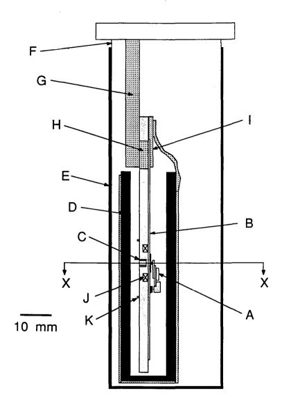
FIG. 2-3. Side view of apparatus. View in Fig. 2-2(b) represented here by section X-X. A is the hot side, B is the sapphire plate, C is the modulation and feedback coil, D is the inner Pb shield, E is the outer Pb shield, F is the vacuum can, G is the Cu tab, H is the Cu disk, I is the clamp, J is the field coil, and K is the big coil. Space constraints allow either the inner Pb shield or the big coil to be mounted, but not both as drawn here.
