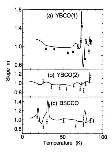
FIG. 5-2. Slope m(T) of noise power spectrum vs. temperature for three samples: (a) YBCO(1), (b) YBCO(2), and (c) BSCCO(1). Points are experimental data. Curves are predictions of Eq. (5-7) from the fits to noise in Fig. 5-1, with  $\tau_0 = 10^{-11}$  s and  $\beta(T) = (1-t^4)/k_BT$ .
