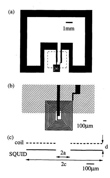
FIG. 6-1. YBCO flux transformer. (a) Pickup loop formed by wide lines, input coil centered on bottom edge, insulating  $SrTiO_3$  layer indicated by dashed box. (b) Enlargement of input coil:  $SrTiO_3$  is shaded region, crossunder is vertical strip connected to center of coil. (c) Cross section of input coil on McDLT hot side placed a distance *d* from Nb-PbIn SQUID on cold side.
