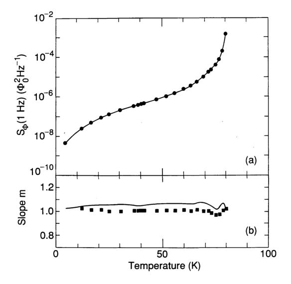
FIG. 5-4. Flux noise from a-axis sample YBCO(6). (a) Spectral density of noise at 1 Hz with SQUID noise subtracted vs. temperature below  $T_c$ . Curve is cubic spline fit to data. (b) Slope m(T) of noise power spectrum vs. temperature. Points are experimental data; statistical error does not exceed height of symbols. Curve is prediction of Eq. (5-7) from the fitted curve in (a), with  $\tau_0 = 10^{-11}$  s and  $\beta(T) = (1-t^4)/k_BT$ . All data points show a 1/f-like noise power spectrum.
