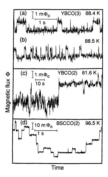
FIG. 3-1. Flux through SQUID vs. time generated by (a) laserdeposited YBCO(3) at 88.4 K, (b) same film at 88.5 K, (c) sputtered YBCO(2) at 81.6 K, and (d) BSCCO(2) flake at 96.5 K. Note changes of scale in (c) and (d). Zeros of axes are arbitrary.
