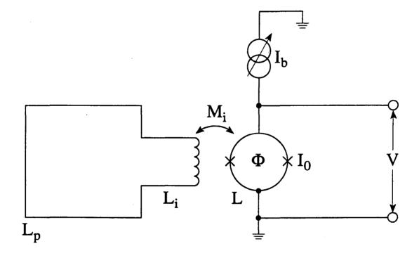
FIG. 1-2. Schematic of dc SQUID of inductance L coupled to superconducting flux transformer. Flux through SQUID is  $\Phi$  and critical current of each Josephson junction is  $I_0$ . Input coil of inductance  $L_i$  has mutual inductance  $M_i$  with SQUID; pickup loop inductance is  $L_p$ .
