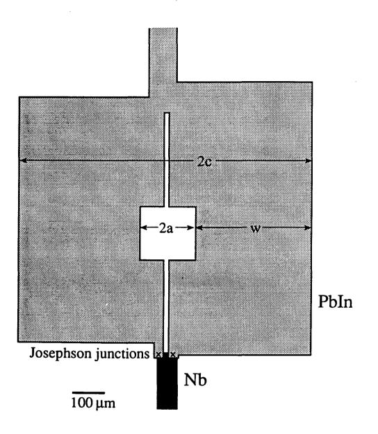
FIG. 2-1. Schematic of thin-film dc SQUID used for flux noise measurements. PbIn square washer has inner radius a, outer radius c, and width w = c-a. Resistive shunts not shown. After Fig. 1.15 of Ref. [81].
