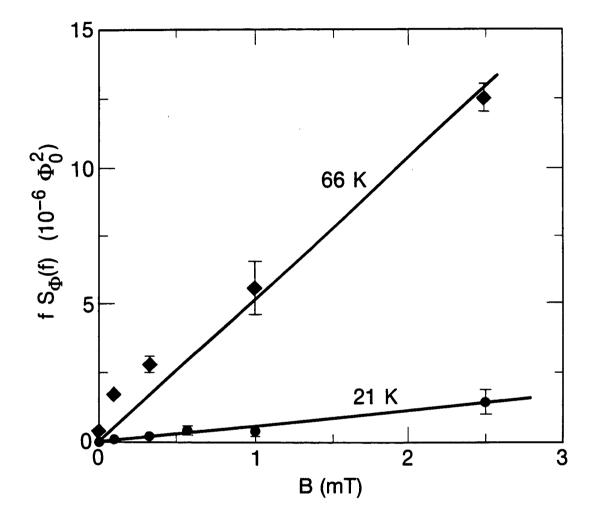
FIG. 8-2. Noise power  $f S_{\Phi}(f)$  for BSCCO(1) at two temperatures as a function of the magnetic field B in which the sample was cooled (1 Hz  $\leq f \leq 100$  Hz). Lines are guides to the eye which intercept the origin.
