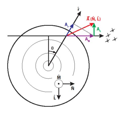
*Figure 11: Coordinate transformation between flux rope's LMN and cylindrical coordinate systems.*
