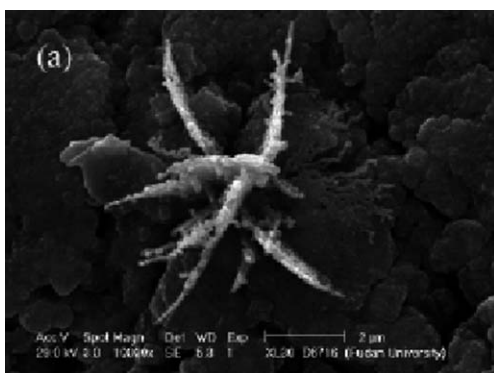
Fig. 12 SEM image of a 3D dendritic morphology formed under self-assembly of \text{Fe}_2\text{O}_3 with application of pyrrolidone as a ligand at 200^\circ\text{C} . Reprinted from ref. 121.
