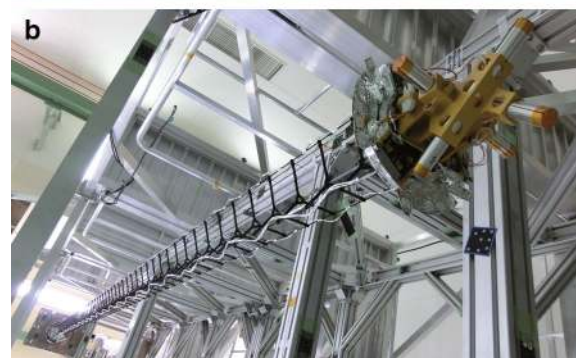
Fig. 5 Photographs of the MSC-S mounted on the top of the MAST in both a stowed and b extended positions. The length of the MAST in full extension is 5.2 m from the side panel of the satellite body
