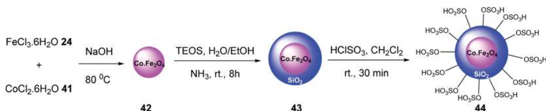
Scheme 12 Synthesis of CoFe 2 O 4 @Silica MNPs 44 .
