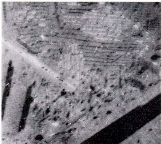
Fig. 3. Titaniferous magnetite from the Mäntyharju gabbroanorthosite. There are thin lamellae parallel to \{100\} between the coarse ilmenite lamellae parallel to \{111\} . These thin lamellae consist of magnetite and extremely small ilmenite lamellae parallel to \{111\} . Polished section, crossed nicols, oil immersion, magn. 800\times Photo, Erkki Halme.
