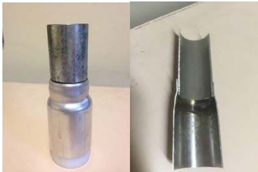
Figure 10 Typical cold welding of stainless steel cylinders.
