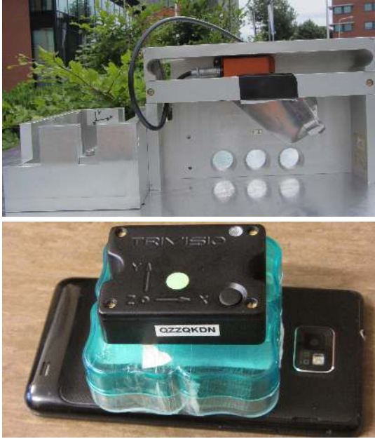
Fig. 2. Top: experimental setup where a calibration experiment is performed outdoors. An Xsens MTi-100 IMU (orange box) together with a magnetic disturbance is placed in an aluminum block. Bottom: experimental setup using a Trivisio Colibri Wireless IMU (black box). A phone is used as a source of magnetic disturbance. To avoid saturation of the magnetometer, the phone is not attached directly to the IMU.
