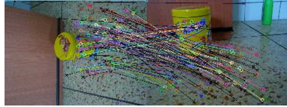
(c) Fundamental matrix; kusvod2 dataset. Errors: \epsilon_{MSC} = 14.3 (2nd) and \epsilon_{MAGSAC} = 0.5 pixels (1st).
