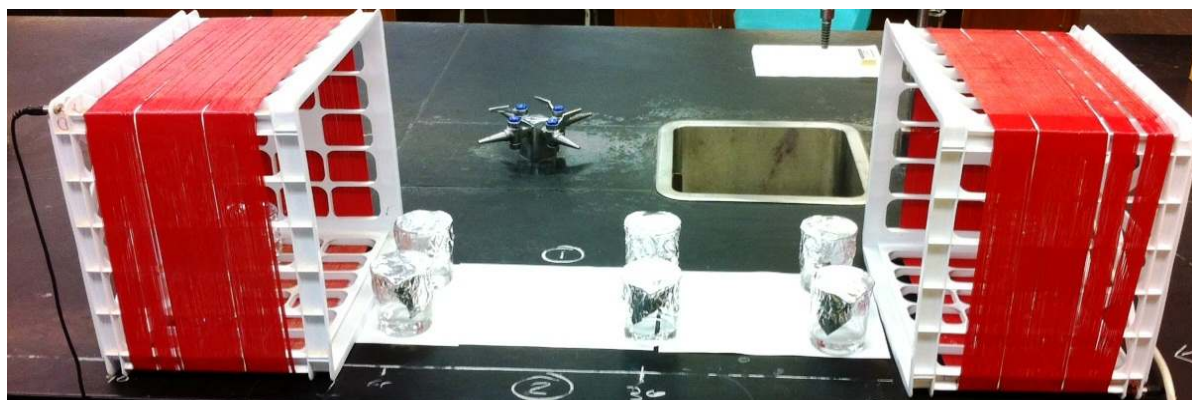
Figure 1. The experimental equipment. When one of the two coils was activated, the proximal containers were location (A), the middle containers were middle (MA), and the distal containers were the non-active (NA). Either coil could be activated.
