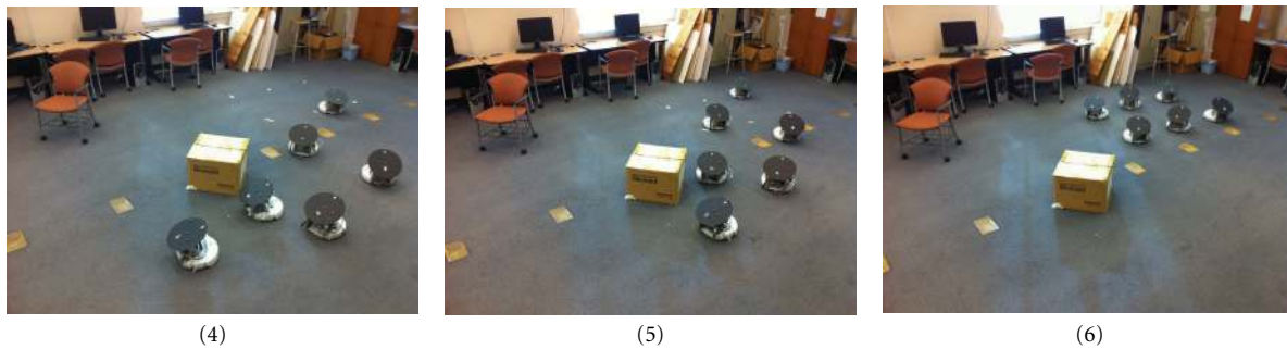
FIGURE 13: Three sequential snapshots of the 6 iRobot Create robots executing the motion planner presented in this paper. Frame 6 is the goal position.
