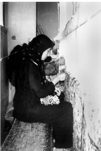
Figure 2. A girl is weaving at a vertical loom. In front of her legs, there is not enough clearance for free leg movements. The seat is a wooden flat piece of lumber without padding.
