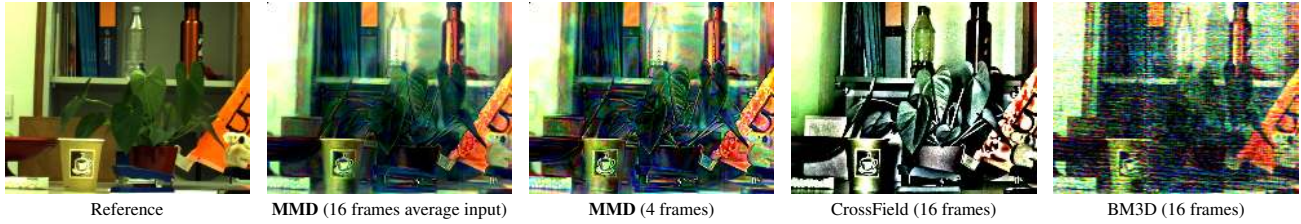
Figure 11: Denoising results for Image 6 (Figs. 6 & 10) in comparison with a reference ‘daylight’ image after applying the same brightness-contrast adjustment operation to each image. The MMD colors come closest to those of the reference image.
