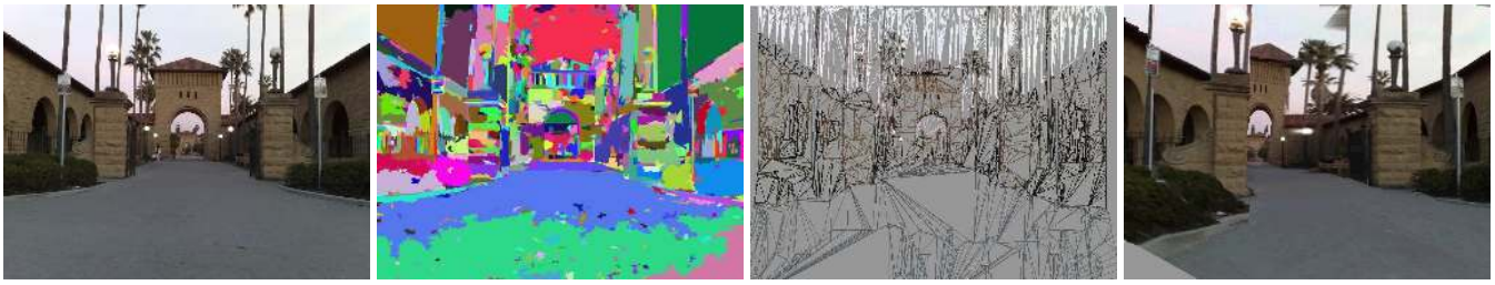
Figure 1: (a) An original image. (b) Oversegmentation of the image to obtain “superpixels”. (c) The 3-d model predicted by the algorithm. (d) A screenshot of the textured 3-d model.
