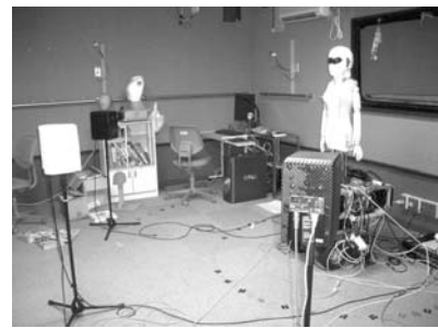
Fig. 5. The room where simultaneous speech signals are recorded on SIG2 .
