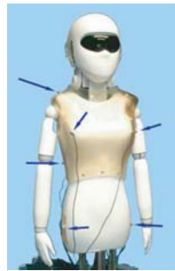
Fig. 4. SIG 2 robot with eight microphones (two are occluded).
