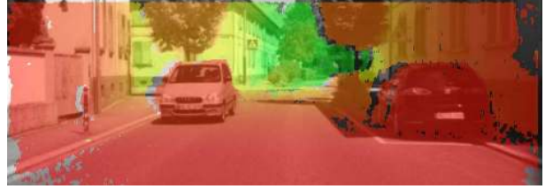
(b) Visualization of the SGM stereo matching result. Red pixels are measured as close to the ego-vehicle ( i.e. dist \leq 10 m) while green pixels are far away ( i.e. dist \geq 75 m).
