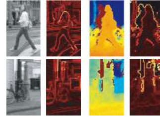
Figure 7: Intensity and depth images with corresponding gradient magnitude for pedestrian (top) and non-pedestrian (bottom) samples. Note the distinct features that are unique to each modality, e.g. the high-contrast pedestrian texture due to clothing in the gray-level image compared to the rather uniform disparity in the same region.
