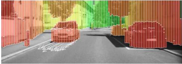
(c) Stixel World representation of the disparity input. Objects are efficiently described using vertical rectangles. The arrows on the base-points of the Stixels show the estimated object velocity. The color encodes the distance.
