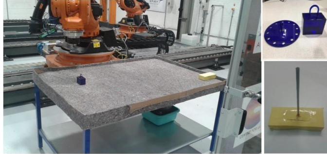
Fig. 3. Workspace table (left) with pick-and-place box (top) and moving obstacle (bottom).
