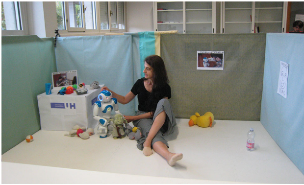
Fig. 2 Robin’s playroom, where the interactions take place. Robin’s toys lie around the room; items including food and the glucometer are on a table. “Family pictures” on the walls are sometimes detected as faces, causing Robin to approach them and open its arms
