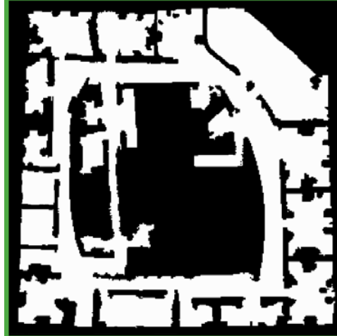
Figure 1: This map of our office was generated by the robot's mapping system
