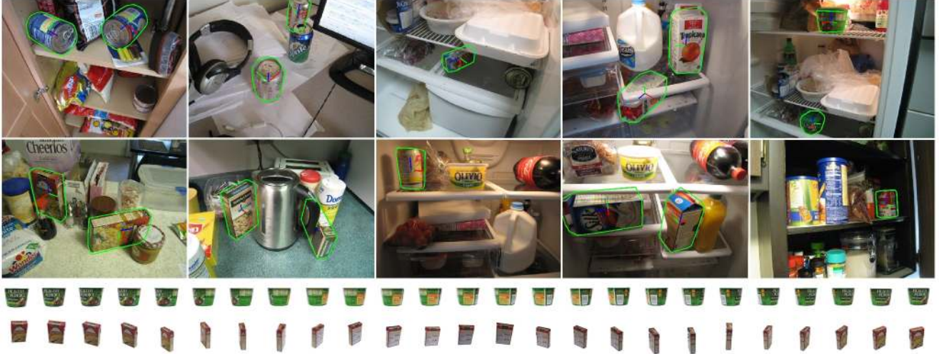
Figure 5. Example detections from our challenging dataset. The images were taken in cluttered environments with different lighting conditions and with the objects under various viewpoints and occlusions. The bottom two rows show the views used to generate the models for two objects.
