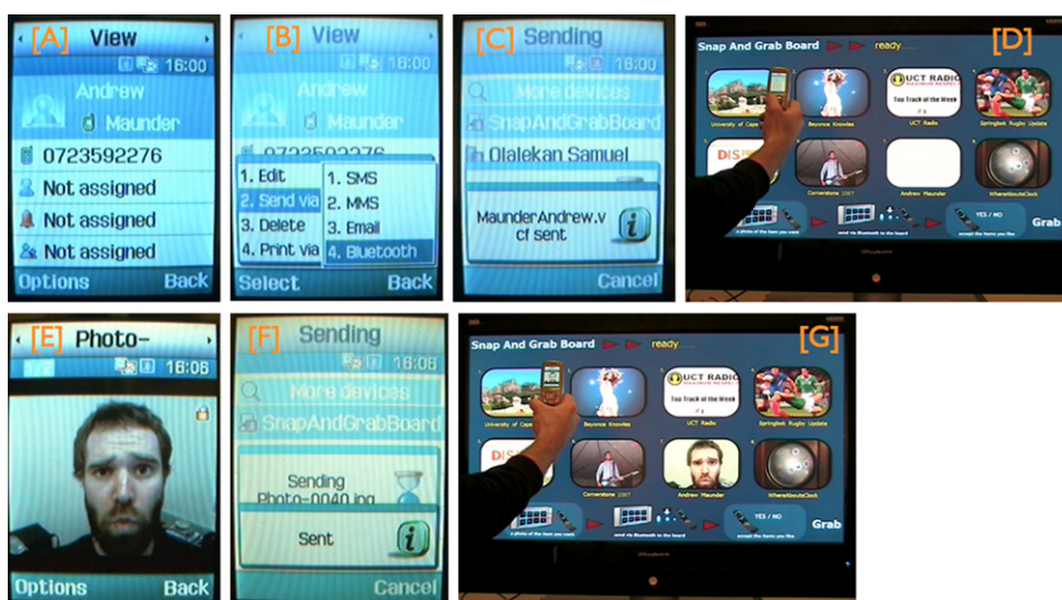
Fig. 2. (A) shows the vCard of the user; (B) shows that vCard being selected for sending; (C) shows the vCard being transmitted to the SnapAndGrabBoard; (D) shows the new, blank, slot being created on the display screen; (E) shows a photo being selected by the user; (F) shows the photo being transmitted to the screen; and (G) shows the photo populating the newly created user-slot.
