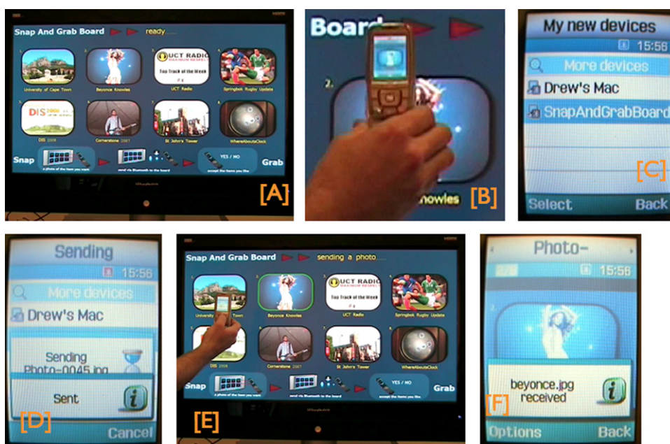
Fig. 1. (A) shows the 40 in. screen; (B) the user takes a picture of the item they are interested in; (C) the ‘SnapAndGrabBoard’ is selected as a target to send the photograph; (D) the photograph is sent; (E) the system performs image recognition on the photograph (feedback is given by highlighting the image in green); and (F) an image (and MP3 in this case) are sent to the transmitting handset.
