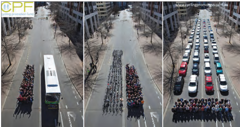
Figure 7.1: Road space required to transport 69 people. (Source: Cycling Promotion Fund, Australia, http://www.bikehub.co.uk/news/sustainability/iconic-waste-of-space-photo-keeps-on-giving .)
