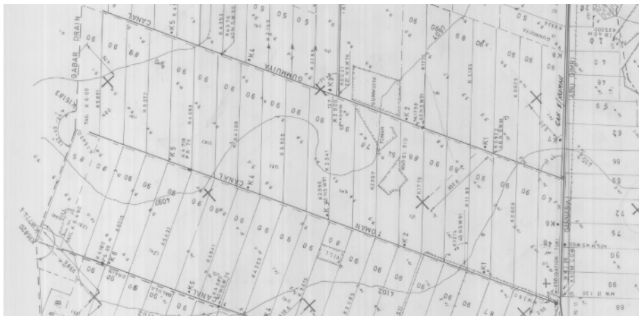
Figure 4.3: Detail of design Drawing Canal layout of Wad Numan Block Nr 4 with layout of Toman canal and villages. Ministry of Irrigation Undated (every rectangle represents 90 acres of land – the total current command area of the scheme is 2.1 million acres). (Source: Ministry of Water Resources, Irrigation and Electricity, Wad Medani Gezira map archive)
