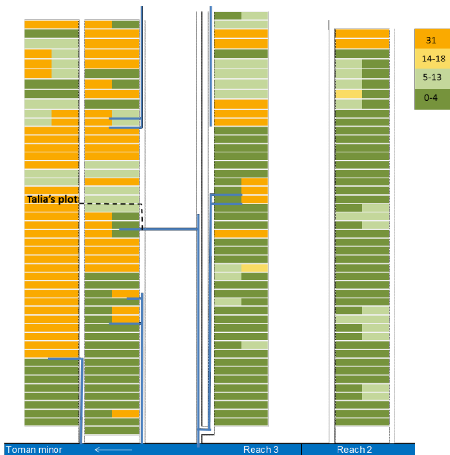
Figure 4.13: Watering status of nimras 10-15 on 4 October 2011 based on field observations. Lines towards plots indicate active irrigation routes. The dotted line is the route Talia is digging. The numbers in the legend indicate the days the plots have been without water.
