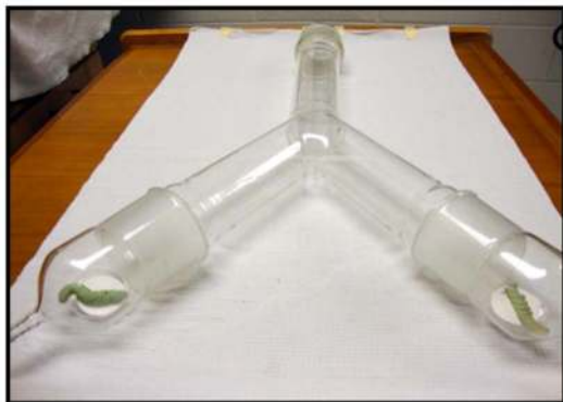
Figure 1. Y-tube olfactometer using live and dead caterpillars. The olfactometer is 70×35×6 cm with the two upwind arms being supplied with charcoal-purified air at a rate of 0.75 litre/sec. doi:10.1371/journal.pone.0108894.g001
