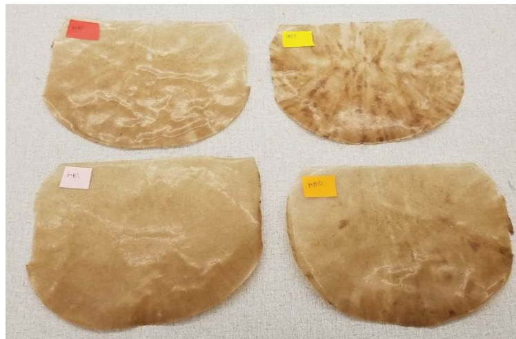
Figure 3.3: Peach flour -high-density polyethylene biocomposites post-compression molding process
