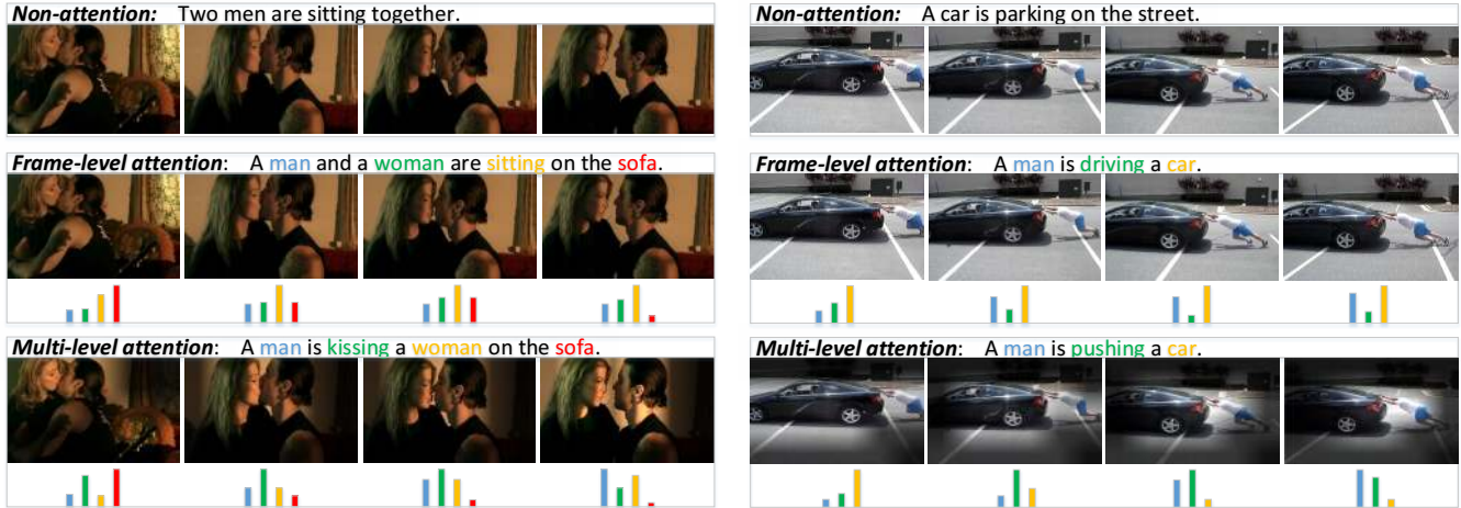
Figure 3: Example results on the MSVD dataset. The sentences above frames denote the captions generated by three variants of our approach, i.e., non-attention, frame-level attention and multi-level attention. The histograms below frames represent the frame-level attention when generating each word (distinguished by color). The brightness distribution in each frame reflects the region-level attention, i.e., the brighter regions are more emphasized.
