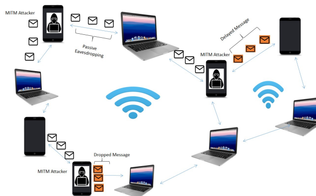
Figure 3. Illustration of both the active and passive modes of MITM assaults in MANET.
