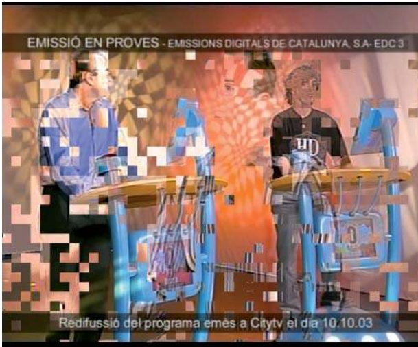
Figure 5. The interference due to man-made impulse noise.
