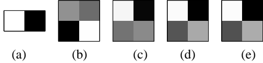
Figure 3. The learned parameters for the 2-class, 5-level MSRF model. The brighter intensity indicates a higher probability. (a) Prior probabilities at the root node (right block indicates the structured class), (b) through (e) transition probability matrices for the links between adjacent levels starting from level 1 to level 5 (top left block indicates the transition from structured to structured class).
