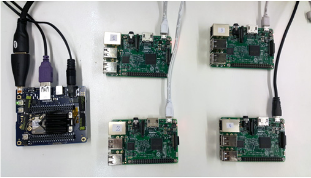
Fig. 6: Embedded computer boards used as controllers.
