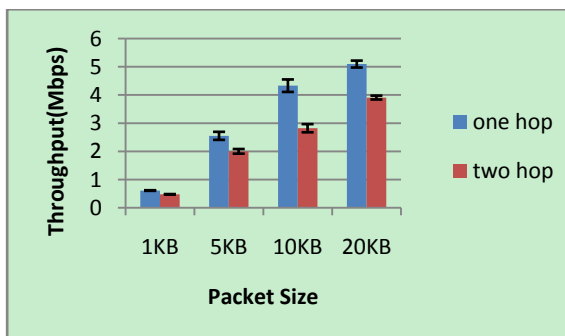
Fig. 9. Average throughput and standard deviation for different packet sizes and number of hops in the 5-meter experiments.
