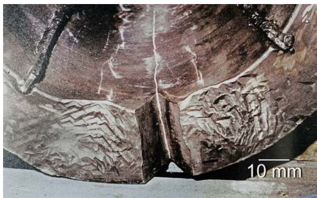
Fig. 11 Arc-gouged notch and a hard region causing a long crack on as-forged nozzle
