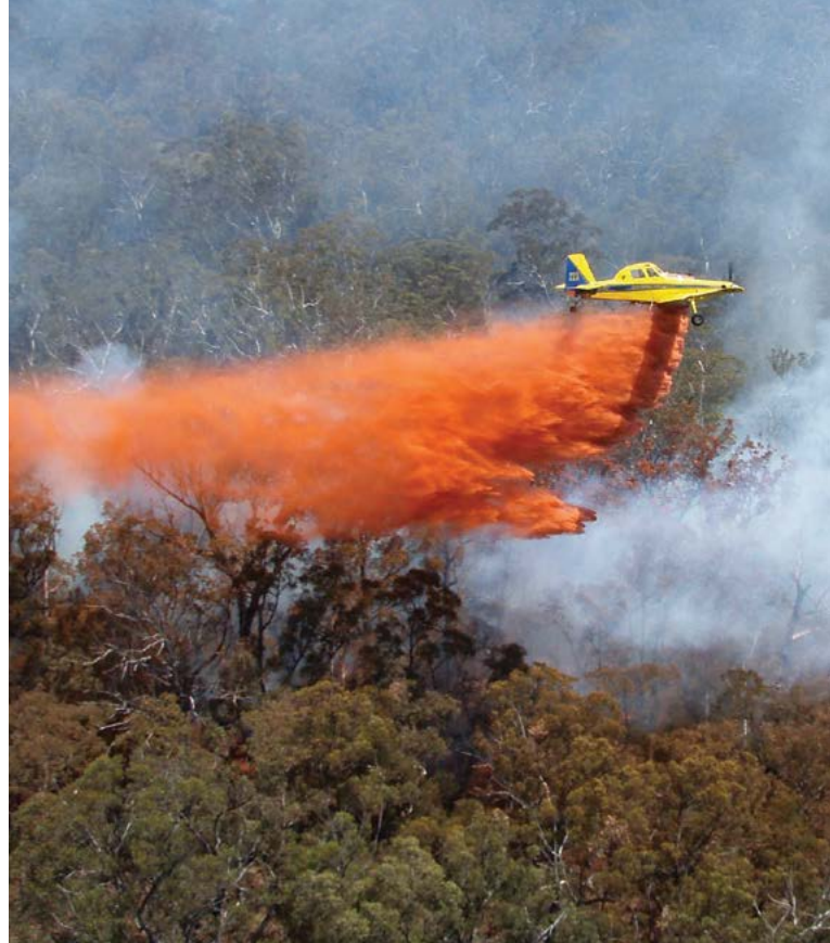
Aerial water bomber spreading fire-retardant chemical (Phos-Chek) to control wildfire, Morton National Park, New South Wales, Australia
