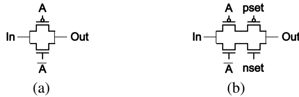
Figure 5.14. Transmission gate design using (a) conventional static CMOS and (b) proposed PTCD methodology.
