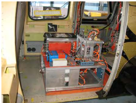
Fig. 4. MicroADAS installation in aircraft.
