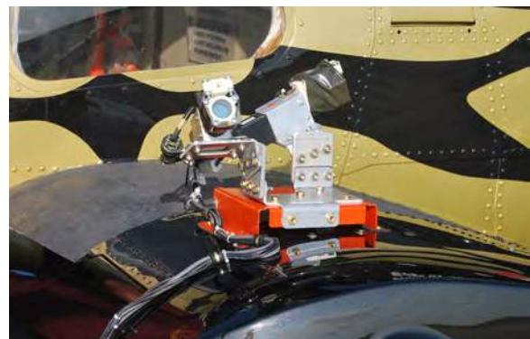
Fig. 7. TPP cameras mounted on pylon.
