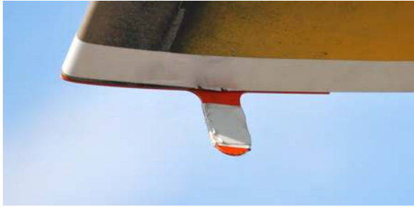
Fig. 8. TPP reflective tape mounted on rotor tip.
