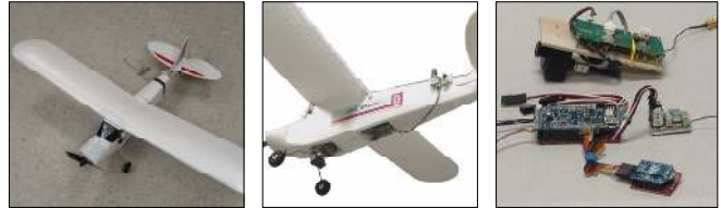
Fig. 10. UAV testbed platform and onboard components
