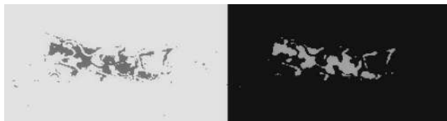
Figure 2. Comparison between the classifications without a majority filter (left) and using a majority filter (right), where it is possible to notice the reduction in isolated pixels and the smoothness of the classified area after applying the filter.
