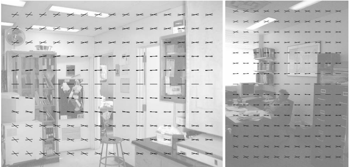
Figure 7: Estimates of the compass angle and geometry obtained by our algorithm. The estimated orientations of the x and y lines are indicated by the black line segments drawn on the input image. At each point on a subgrid two such segments are drawn – one for x and one for y . Left panel: Observe how the x directions align with the wall on the right hand side and with features parallel to this wall. The y lines align with the wall on the left (and objects parallel to it). Right panel: Observe that the x, y directions align with the appropriate walls despite the poor quality of the image (i.e. under-exposed).
