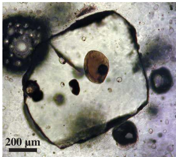
Fig. 2. Photomicrograph of an olivine-hosted melt inclusion. The inclusion pictured is sample GUG-D, from Guguan island. The olivine crystal is embedded in resin and has been polished to expose the melt inclusion at the surface. The inclusion is made of clear, brown glass and contains a single vapor bubble.
