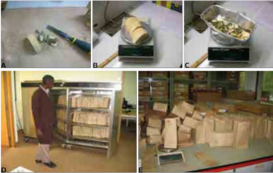
PHOTO 3.8 – Laboratory measurements: (A) debarking, (B) weighing the wood, (C) weighing the bark (photos: L. Saint-André), (D) oven-drying samples, (E) regular weighing to constant weight (photos: M. Henry).
