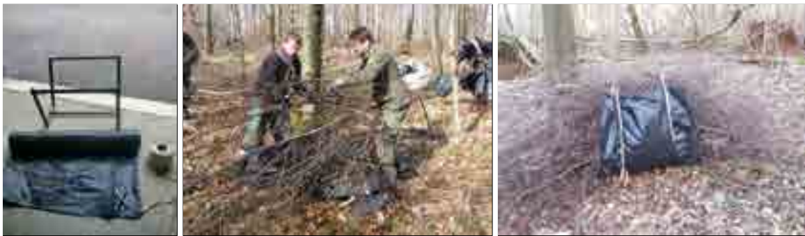
PHOTO 3.14 – Bundling branches. Left, iron frame, tarpaulin and string for bundling branches (photo: A. Genet); middle, bundling branches in the field (photo: M. Rivoire); right, bundle ready for weighing (photo: M. Rivoire).
