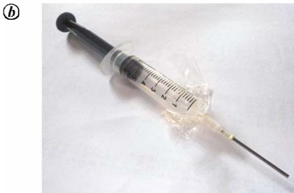
Figure 2. a, Schematic diagram of the Reddy tube. b, Photograph of a medical syringe converted into piston-driven mini shock tube.
