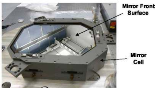
Figure 9. FM2 installed in cell.
