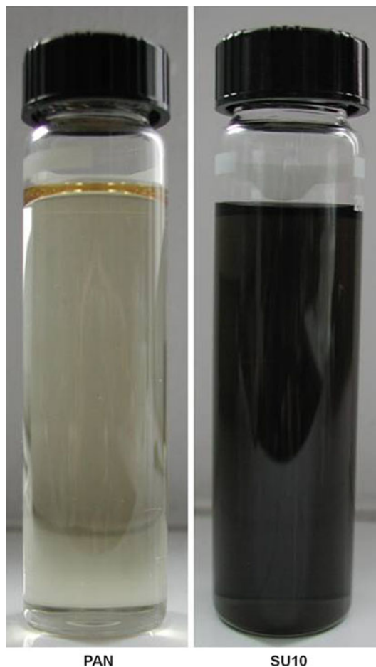
Fig. 5 Pure PAN solution and PAN suspension containing SWCNH after optimisation process
