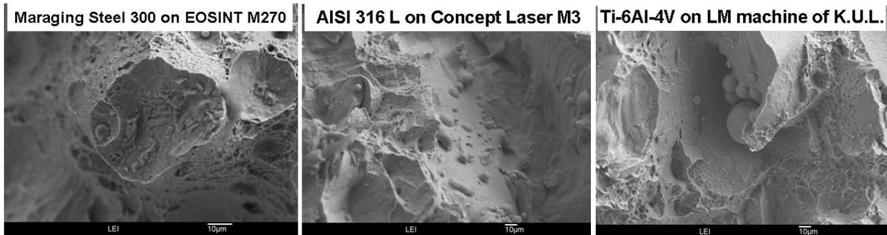
Figure 5.50: Un-melted powder particles in the pores of all samples produced on different machines
