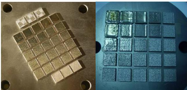
Figure 4. Parts made for parameter study for laser surface remelting; stainless steel on the left and Ti-6Al-4V on the right.
