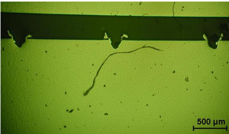
Figure 2.27: Laser marks made with 10 mm/s, 39 A, 5 kHz and big aperture
