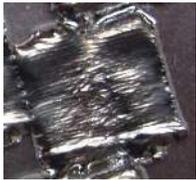
Figure 34. Large deformations of a part remelted with a power of 300 W, a beam diameter  $\Phi_{1/e^2}$  of 100  $\mu\text{m}$  and a scan speed of 20 mm/s.
