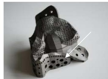
Figure 1: SLM part with cracks induced by thermal stresses.
