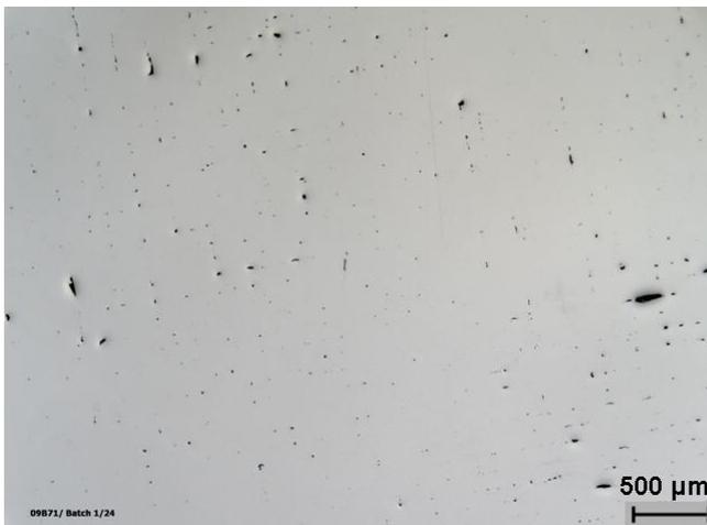
Figure 5.69: Optical micrograph taken perpendicular to the building axis (*xy*-plane) without re-melting (melting with  $a_2= 30\%$  and  $a_1= 70\%$ )
