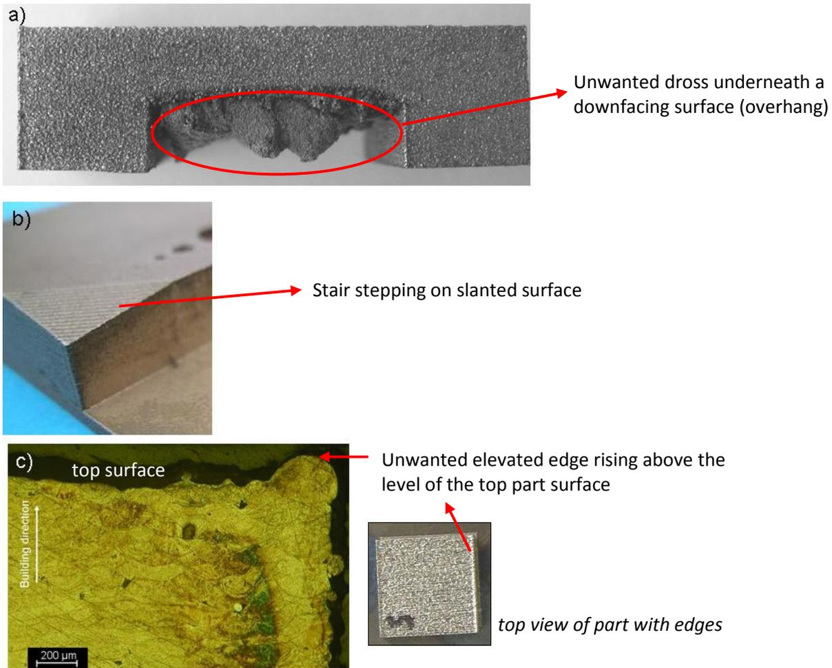
Figure 1.3: a) Excessive dross formation due to local overheating in an overhang structure b) stair stepping effect c) elevated edges formed during SLM
