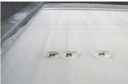
Figure 3.39: Top of the powder bed showing the expelled powder
