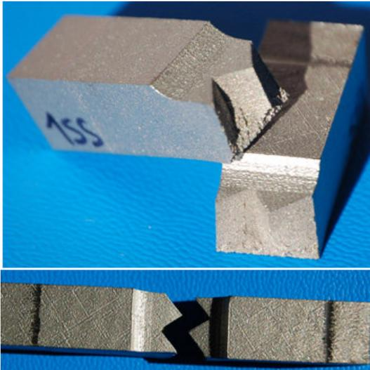
Figure 5.35: AISI 316L parts produced on a Concept Laser M3 Linear with island scanning and insufficient overlapping between islands
