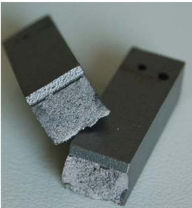
Figure 5.44: Fracture surface of maraging steel standard specimens
