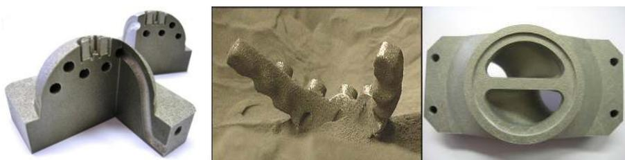
**Figure 1** Sample parts produced by SLM
