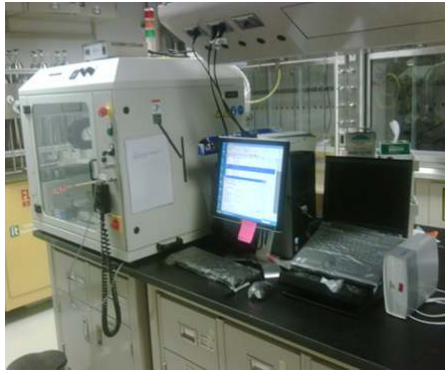
Figure 1.49. Sono-spray deposition system for nanoparticle thin film processing (L) and Perkin-Elmer Lambda 900 spectrophotometer with integrating sphere attachment (R)
