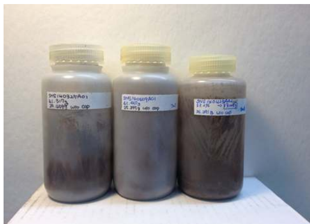
Figure 1.36. Samples produced from the low temperature materials synthesis project. The material was > 50g of SnS and was oxidized to n-type SnO 2 and used for gas sensing.
