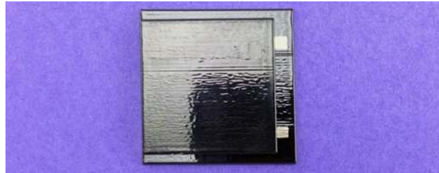
Figure 2.15. A prototype embedded strain gauge. Inkjet printed silver between two 1-mm thick FDM layers.
