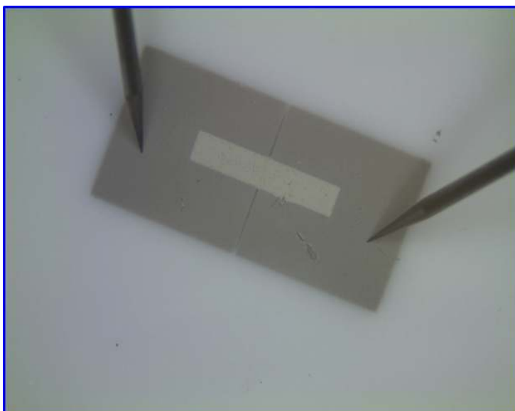
Figure 3.34. SnO 2 screen printed between two Pt pads.
