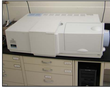
Figure 1.49. Sono-spray deposition system for nanoparticle thin film processing (L) and Perkin-Elmer Lambda 900 spectrophotometer with integrating sphere attachment (R)
