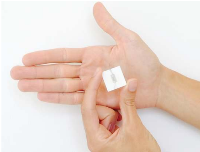
Figure 3.38. ZnO sensor made from 1 mm wide strip of screen printed ZnO on Alumina substrate. The electrodes were screen printed Pt 100 \mu\text{m} .
