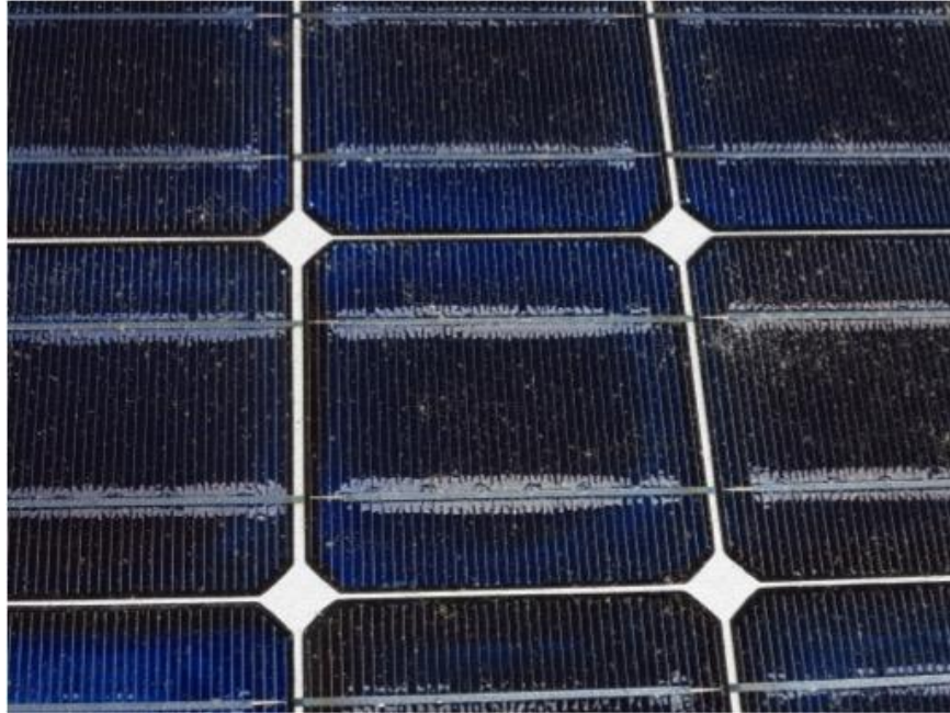
Figure 7. Image of module with delamination of the encapsulant near the busbars on each cell.
