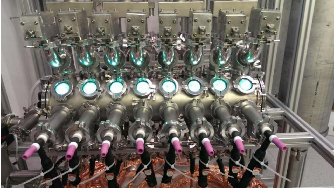
Figure 1. Multiple optimized single units of BUONAPART-E's project for large scale production of metal nanoparticles by using electrical discharge methods.
