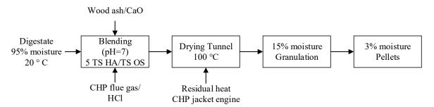
**Figure 7.** Proposed process A for the manufacturing of a granular fertilizer. (CHP = Combined heat and power plant) to be implemented at the headquarter of a 40,000 tonnes/year production facility of anaerobic digestate with a CHP unit for valorization of the biogas. Optimum blending ratio was defined as 5 TS HA/TS OS [31].
