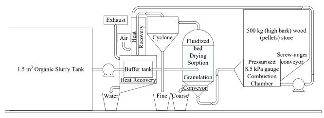
**Figure 4.** Modified wood pellet boiler for processing 1 tonne of fresh OS (95% moisture) in a 10 h batch operation, consuming 180 kg of wood pellets [94]. The granular organic amendment (51 kg) contains 0.03% of wood ash, in addition to the dried manure (99.97%). Inspired in the media slurry drier of Nara Machinery Ltd. (Tokyo, Japan) [95].
