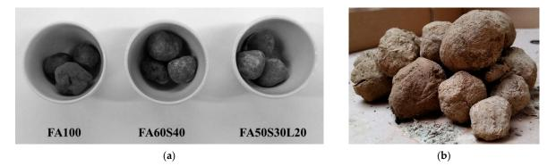
**Figure 3.** (a) Granular fertilizer (10 mm diameter) prepared by Pesonen et al. [78] with 100% fly ash, 60% fly ash and 40% sludge, and 50% fly ash, 30% sludge and 20% lime  $(Ca(OH)_2)$ . Reprinted with permission of the Journal of Environmental Chemical Engineering (Elsevier). (b) Granular fertilizer (greatest diameter around 30 mm; 3% moisture) prepared during the OWAS project, involving only the step of physical stabilization of anaerobic digestate (80%) with wood ash (20%).
