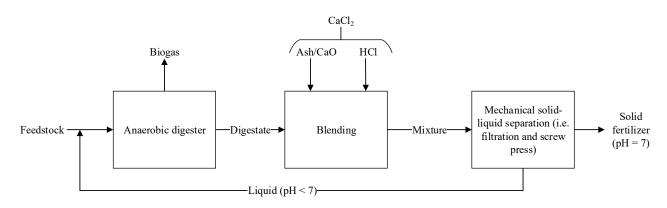
**Figure 8.** Proposed process B to be implemented directly at the anaerobic digestion plant of one of the stakeholders of the OWAS project.
