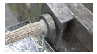
Fig. 11.5 Composites before entering heated die (Courtesy of Rasidin Senawi of Innovative Pultrusion Sdn. Bhd., Seremban, Negeri Sembilan, Malaysia)
