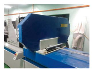
**Fig. 11.9** A cutter in a pultrusion machine (Courtesy of Rashidin Senawi of Innovative Pultrusion Sdn. Bhd., Seremban, Negeri Sembilan, Malaysia)
