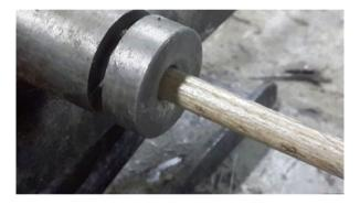
Fig. 11.7 Fully cured pultruded composite after leaving the heated die.(Courtesy of Rasidin Senawi of Innovative Pultrusion Sdn. Bhd., Seremban, Negeri Sembilan, Malaysia)
