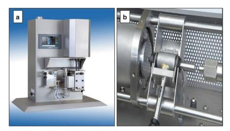
Fig. 14.3 (a) Micro-compounder and (b) micro-injection molding machine
