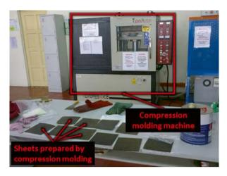
Fig. 1.3 Hot Compression moulding machine (Courtesy of Y.A. El-Shekeil)
