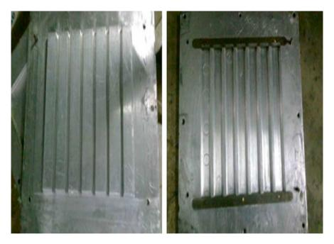
Fig. 15.5 Pictures of mould used for composite manufacturing
