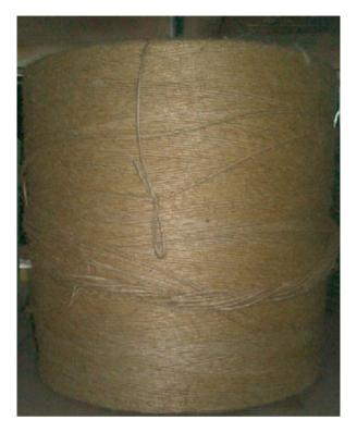
Fig. 18.4 Kenaf yarn fibre
