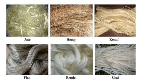
Fig. 2.2 Images of plant-based fibres
