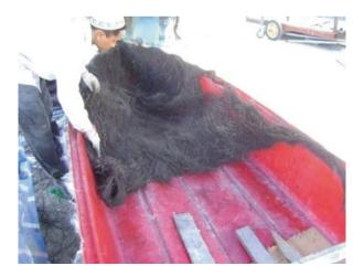
Fig. 1.2 Hand lay-up process for hybrid glass-sugar palm composite boat (Courtesy of S. Misri)
