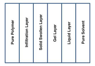
Fig. 16.3 A schematic of the composition of the surface layer (adapted from Miller-Chou and Koenig 2003)
