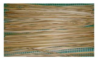
Fig. 10.2 Extracted puchika grass by pure splitting method
