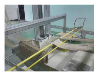
Fig. 1.1 Pultrusion process of kenaf fibre fibre composites (Courtesy of A.M. Fairuz)
