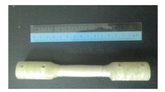
Fig. 18.3 Shaft made from filament winding process
