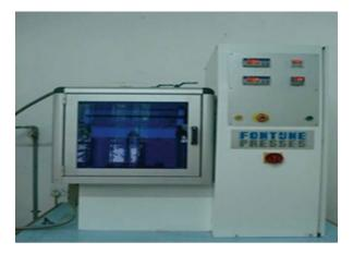
Fig. 15.2 Hot compression moulding machine
